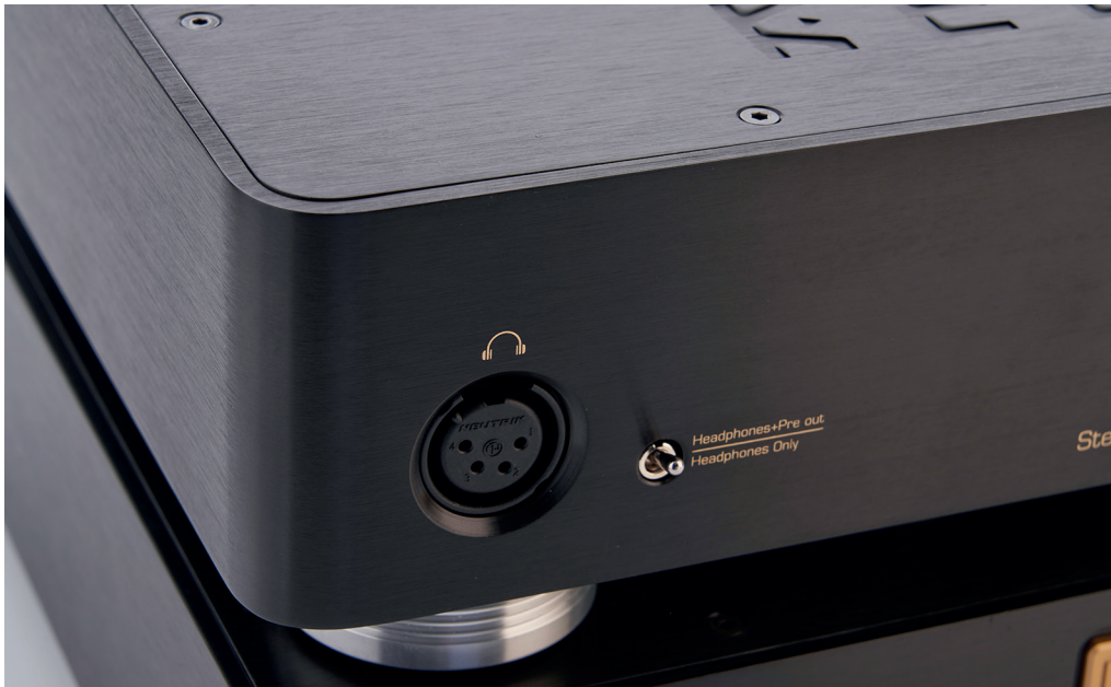
For headphones, the KECES has on offer only this four-pin XLR socket, which is common for balanced outputs
